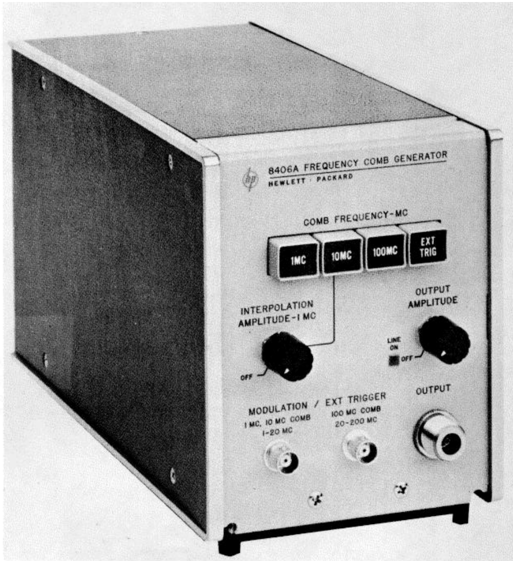
Figure 1-1. Frequency Comb Generator
